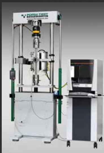
Example for servo-hydraulic test machine
