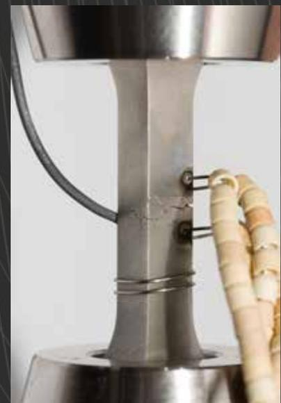
Example of the application of a potential drop probe (\*)
