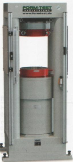
Fig. 2 Compressive testing machine frame.
